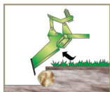
The Shock Control goes into action and disarms the rod.
